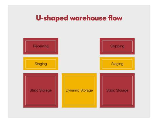
The intention of the U shape is to keep major warehouse traffic flow separate to avoid bottlenecks. This flow of goods assists in minimising the available space required and fits into many warehouse buildings as both the entrance and the exit share the same side of the building. The other benefit is that less space is needed for packages, and warehouse staff can quickly move products between receiving and shipping areas.
