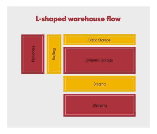
The L shape layout has the shipping area at a 90-degree angle to the receiving area. The warehouse building requires a larger space for this layout to operate, as it is uncommon to have doorways located to match this floor plan.
