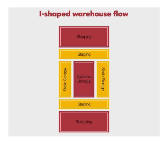
The I-shape warehouse design operates with a straight flow from the receiving area to the shipping area and vice versa. This setup is said to maximise optimisation as it utilises the entire length of the warehouse. The layout can be easily expanded in static storage design areas. The layout also separates similar products in an assembly-line format and reduces potential bottlenecks through back-and-forth inventory movements.
