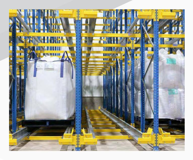
The remote-controlled pallet shuttle is a self-powered device that runs on rails in the storage channels for retrieving pallets. The system carries goods in and out of deep storage tunnels without any human intervention. It is an excellent solution for long term or dense storage of a large number of pallets using a minimal building footprint. Using this automation solution delivers low running costs but does require highly efficient warehouse management.
